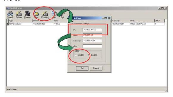
Step4: After modify to IP and DHCP function of the I-7540D, it will reboot automatically. And the DHCP function of the I-7540D will be disabled. (2011/02/08,Andy)
